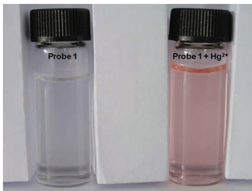
Figure 1. “Naked-eye” color changes of probe 1 ( 20\ \mu\text{M} in pure water) before and after addition of \text{Hg}^{2+} ( 1.0\ \mu\text{M} ) at room temperature (reacted 15 min and adjusted pH to 7.4 with PBS buffer before measurement).
